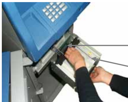
Fig. 5.3a Replenishing the Cash Cassette
